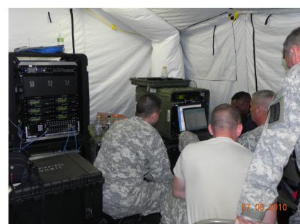
the JFHQ-NY-J6 Tactical Communications Team training on the rack of radios in the Voice Interoperability Modular (VIM). The VIM can program the frequencies used by first responders across all spectrums into the JISCC radio network for full interoperability to support Command Control Communications and Computers (C4) at an incident site.
