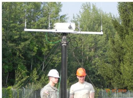
SGT Kevin Grabowski and SSG David Colliton JFHQ-NY-J6 as they are preparing to erect the antenna for the Voice Interoperability Modular (VIM). The antenna supports the VIM which is used to scan and identify emergency responder frequencies broadcasted in a disaster area.
